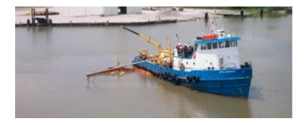
The VOSS (yellow) is being deployed and connected to an out-rigged arm. This is suitable for collection in both large pockets of oil and for recovery of streaming oil. The oil-to-skimmer encounter rate is limited by the length of the arm. Skimming pace is  $\leq 1$  knot.
